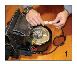
Put fully charged battery in blower pack and connect to blower.
